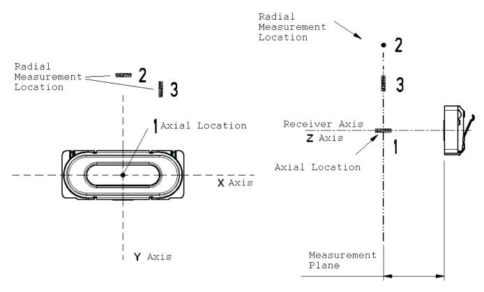
Axial (position 1): maximum value of Z direction Radial X (position 2): maximum value of X direction
