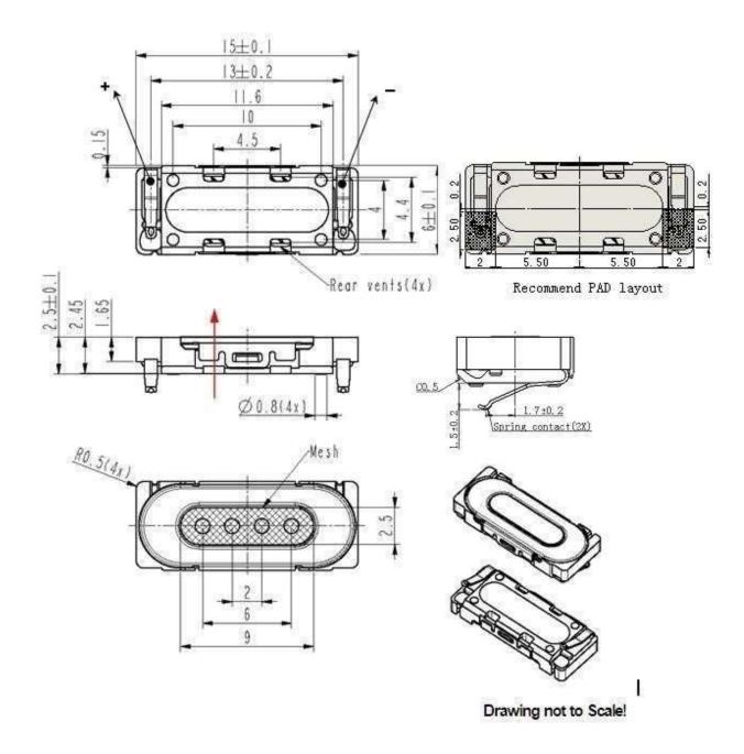
Positive voltage on pad '+' moves membrane in direction of red arrow!
